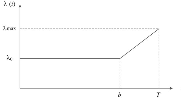
Fig. 1. Example of the stream of damages of ageing elements
